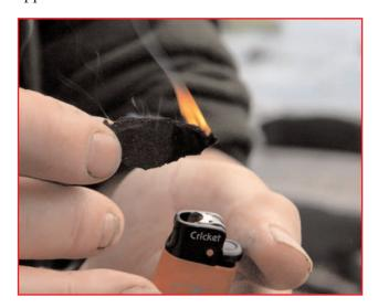
Setting light to oil shale at Clavels Hard east of Kimmeridge
